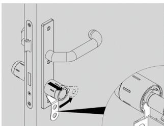
Fig. 18: Removing the knob sleeve
